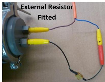
Once water conductivity has been brought back to the correct level the resistor can be removed. Leaving the resistor in place will not however, damage or affect the efficiency of the Aligator.
